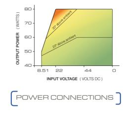
CAMSWITCH 4 Mobile can operate from an 8.5V
