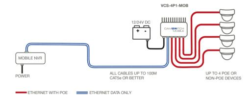
CAMSWITCH 4 Mobile delivers a network connection and optional POE to 4 cameras. POE is converted to IEEE 802.3af / 802.3at levels from a 12V or 24V DC supply.
